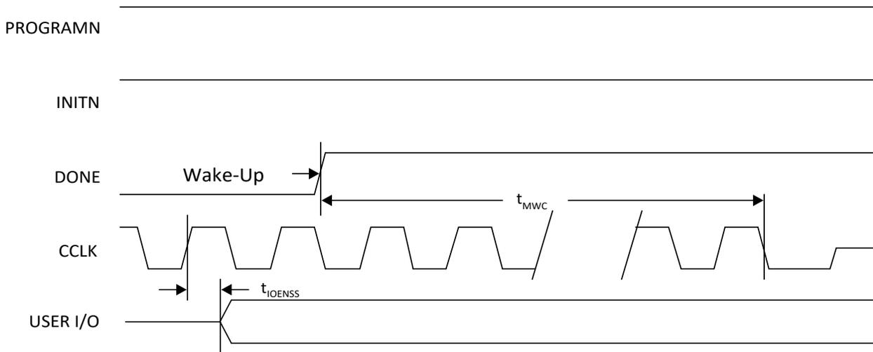
**Figure 3.21. Wake-Up Timing**
