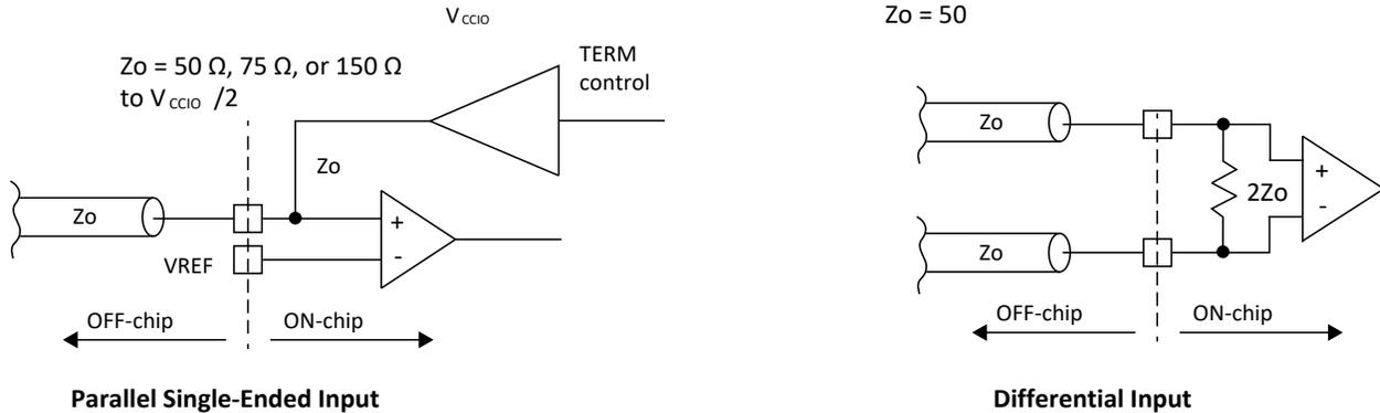
Figure 2.26. On-Chip Termination
