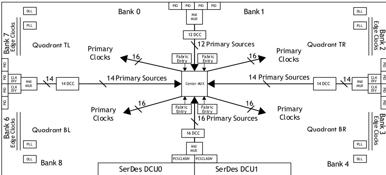
**Figure 2.6. LFE5UM/LFE5UM5G-85 Clocking**
