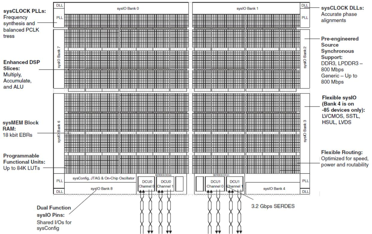
**Figure 2.1. Simplified Block Diagram, LFE5UM/LFE5UM5G-85 Device (Top Level)**
