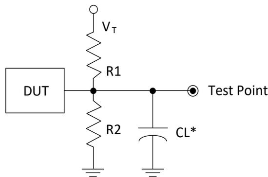
\*CL Includes Test Fixture and Probe Capacitance
