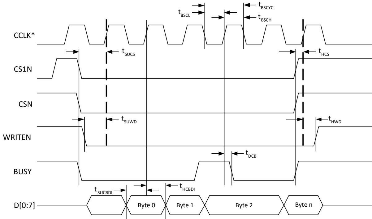
\*In Master Parallel Mode the FPGA provides CCLK (MCLK). In Slave Parallel Mode the external device provides CCLK.
