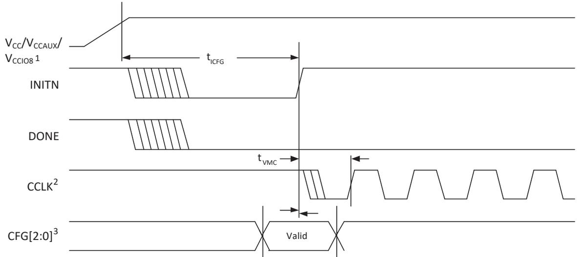
1. Time taken from  $V_{CC}$ ,  $V_{CCAUX}$  or  $V_{CCIO8}$ , whichever is the last to cross the POR trip point.
