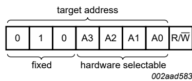
Figure 7. PCA9575 device address for 28-pin version
