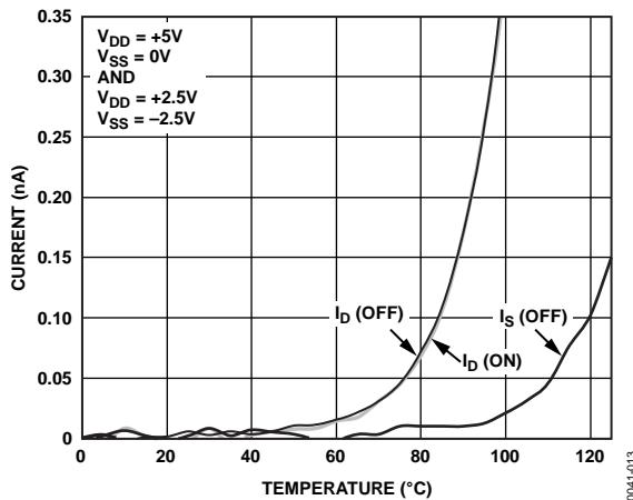
Figure 13. Leakage Currents as a Function of Temperature
