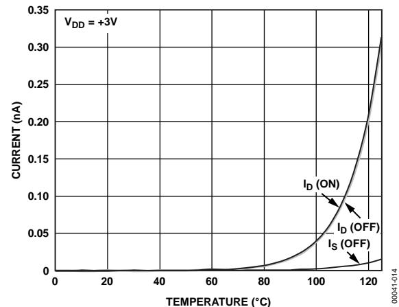
Figure 14. Leakage Currents as a Function of Temperature
