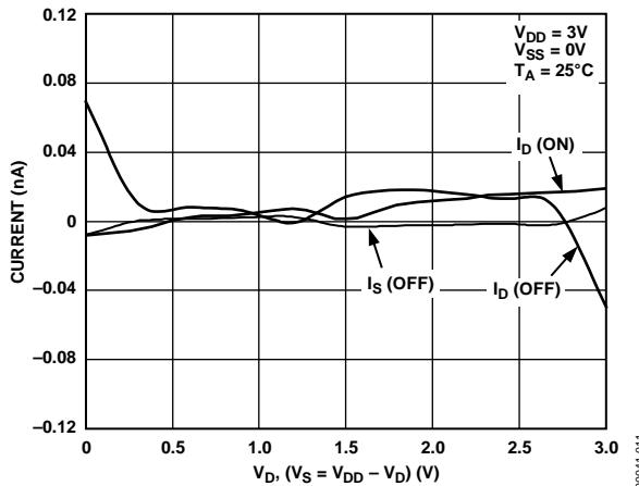
Figure 11. Leakage Currents as a Function of  $V_D$  ( $V_S$ )
