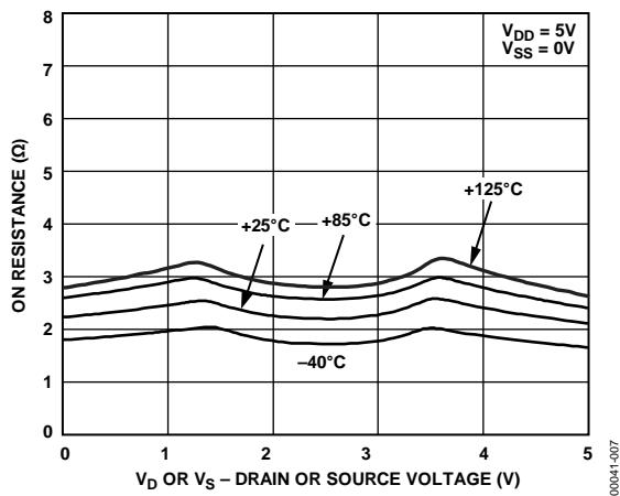
Figure 7. On Resistance as a Function of  $V_D$  ( $V_S$ ) for Different Temperatures, Single Supply
