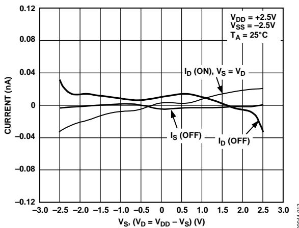
Figure 12. Leakage Currents as a Function of  $V_D$  ( $V_S$ )
