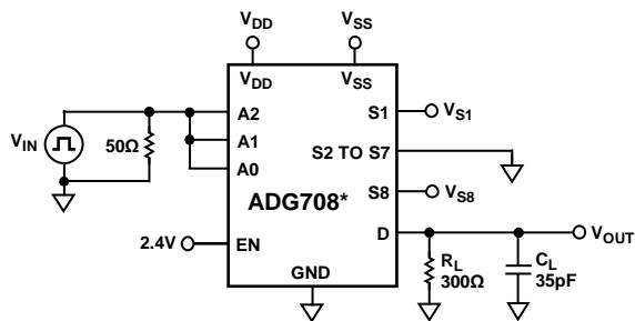
Figure 24. Switching Time of Multiplexer,  $t_{TRANSITION}$
