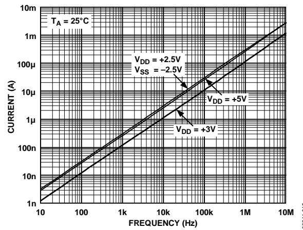
Figure 15. Supply Current vs. Input Switching Frequency
