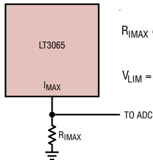
$$R_{IMAX} = \left( \frac{600mV}{I_{OUT(MAX)}} \right) \cdot 500$$
