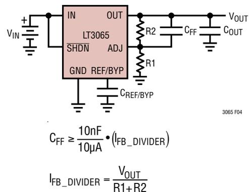
**Figure 4. Feedforward Capacitor for Fast Transient Response**
