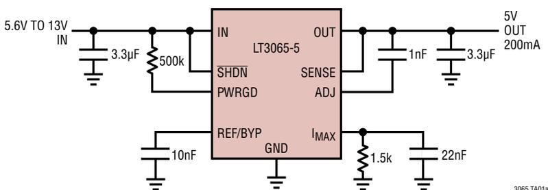
**Precision Current Limit,  $R_{I_{MAX}} = 1.5k$**
