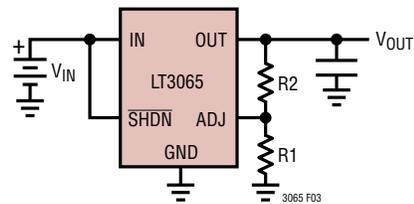
$$V_{\text{OUT}} = 0.6\text{V} \left( 1 + \frac{\text{R2}}{\text{R1}} \right) - (I_{\text{ADJ}} \cdot \text{R2})$$
