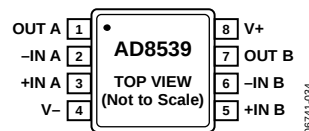
Figure 4. 8-Lead MSOP (RM-8)
